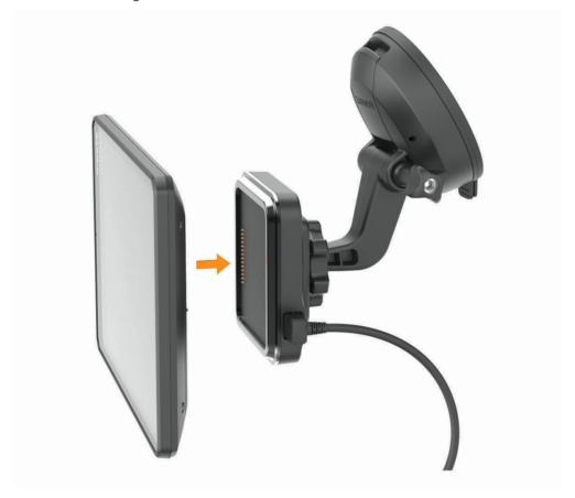
6 Plug the other end of the vehicle power cable into a power outlet in your vehicle.
