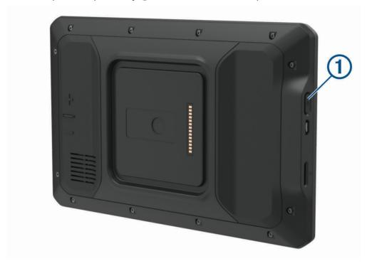
To put the device in power saving mode, press the power key while the device is on.
